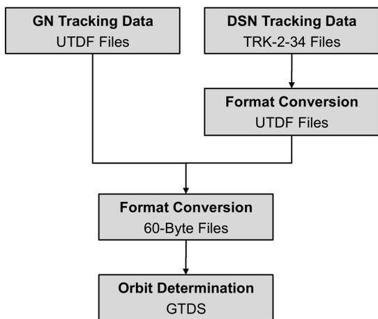
**Figure 5. Pre-processing flow for radiometric range and range rate tracking data.**
