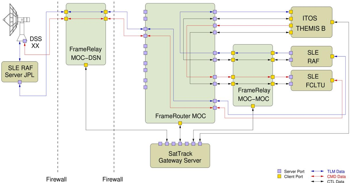
**Figure 2. Network routing scheme for bidirectional telemetry and command flows across socket connections using the SLE protocol, shown in this example for THEMIS B. The overall architecture allows concurrent passes with all five probes across all mission networks, with and without the SLE protocol.**
