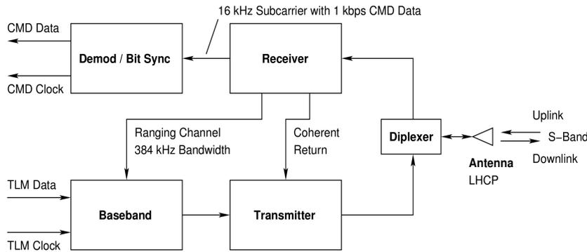
**Figure 4. THEMIS S-band phase-locked transponder block diagram.**
