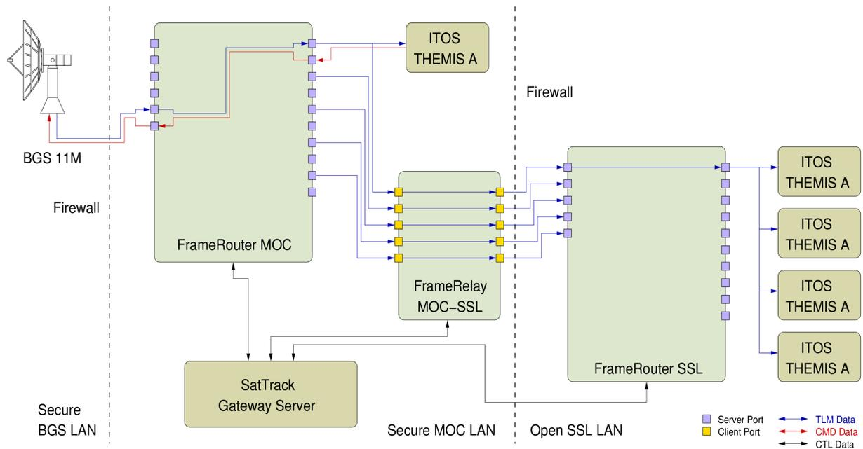
**Figure 1. Network routing scheme for unidirectional telemetry and command socket connections.** Example shown for THEMIS A real-time telemetry and telecommand data flows between the Berkeley Ground Station and the primary ITOS command and control workstation. Telemetry data are also routed to additional ITOS workstations outside the MOC to allow remote monitoring of spacecraft state-of-health to support special operations.
